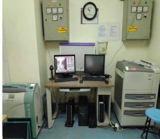
Gambar 4.9 Processing Unit Computer Radiografi
